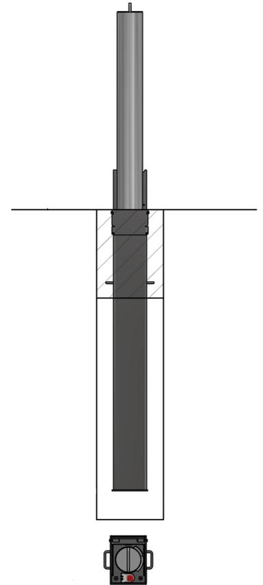
The RetractaPost-GL offers a highly effective and robust way to protect premises and vehicles. The RetractaPost-GL is raised and lowered vertically. When raised the post is 745mm above ground, when lowered the post is fully below ground and covered using the integral lid. The post is lockable in the raised position by rotating the post 45° and then pressing the high-security push button 7-pin security lock. The post is unlocked using the supplied key, rotated and then lowered.
