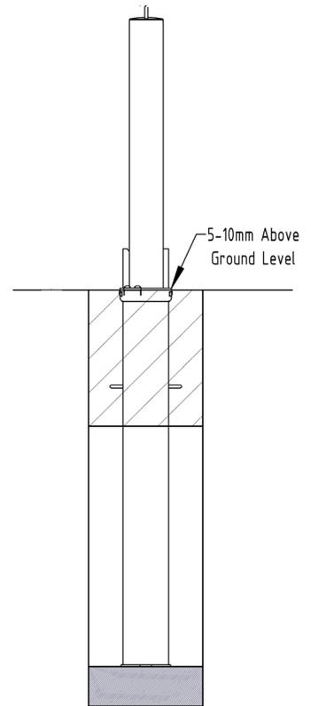
The RetractaPost FB is a simple, cost effective, yet highly effective way to prevent unwanted vehicle access. The RetractaPost FB is raised and lowered vertically. When lowered the post is fully below ground and covered using the integral lid. The post is padlockable (padlock not supplied) in the raised position by first rotating the post 45° and then attaching the padlock between the post to the lid.
