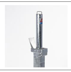
The RetractaPost is a simple, cost effective, yet highly effective way to prevent unwanted vehicle access. The RetractaPost is raised and lowered vertically. When lowered the post is fully below ground and covered using the integral lid. The post is padlockable (padlock not supplied) in the raised position by first rotating the post 45° and then attaching the padlock between the post to the lid. The RetractaPost 500 is 500mm above ground in the raised position.
