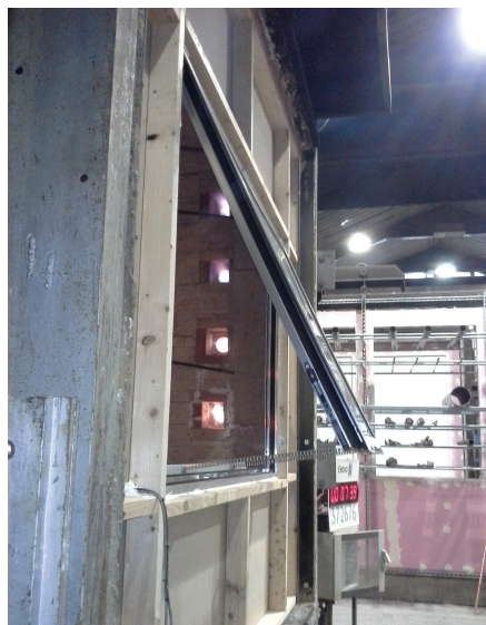
Smoke vent in test chamber
