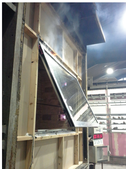
Smoke vent Annex G testing almost coming to an end at the 30-minute mark
