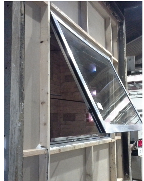
Smoke vent with twin chain actuator
