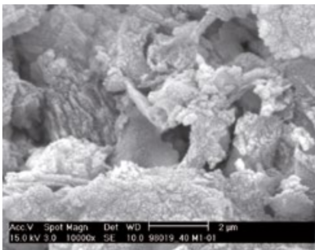
PHOTO 3 - Micrograph of ancient mortar. Notice how the amorphous mass is completely carbonated
