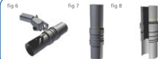
The pipe connecting into the ring seal adaptor should be inserted fully into the socket and marked. To create the expansion gap withdraw the pipe 12mm from the socket. This gap will allow the pipe to expand sufficiently without distorting the pipework. (figs 6,7&8)
