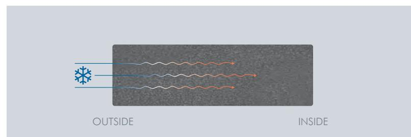
Sealing tape without microtherm technology
