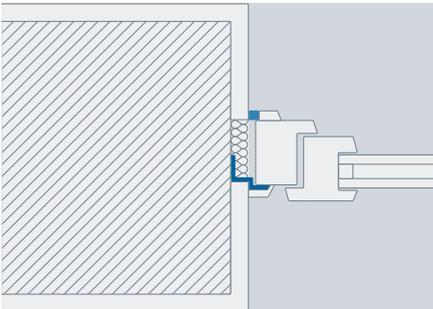
Level reveal at the side (monolithic masonry)
