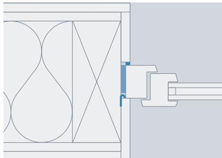
Level reveal at the side (timber-frame construction)
