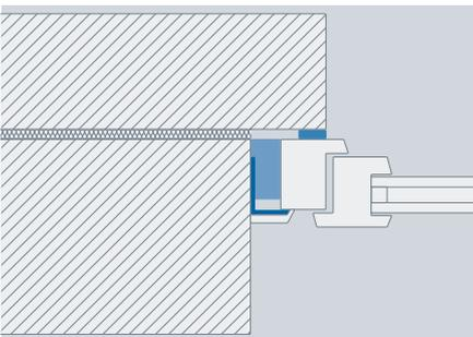
Check reveal at the side (double-wall masonry)
