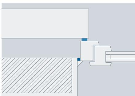
Check reveal, faced with brickwork / block work
