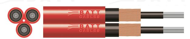
These utility mains power cables, arranged in triplex formation with three single cores, and manufactured to BS 7870-4.10 standards, are designed for efficient power distribution. Commonly used by Distribution Network Operators (DNOs) and generation utilities, they are ideal for connecting electrical grids to sub-main developments and are suitable for power networks, outdoor installation, and cable ducting.
