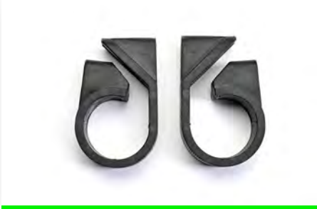
Telcleat Single-piece, single-fixing cleats made from low-density polyethylene. UV and weather resistant. Suitable for cables with outside diameters of between 10mm and 51mm.
