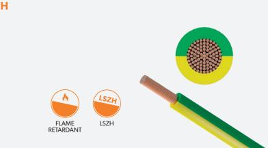
Single core LSZH cable used in fixed wiring protected installations. Available as standard in sizes up to 630mm<sup>2</sup> and in 11 insulation colours. BASEC Approved.
