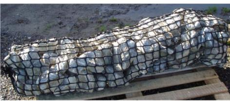
Rock Rolls that are installed below coir units can also be used to support a filter fabric or biodegradable matting. This system retains the fines in the bank while the roots of the plants from the pre-vegetated coir units establish themselves into the bed of the waterway and through the woven geotextile into the suitable fill.
