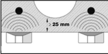
1. Locate rebars by means of suitable detector.
