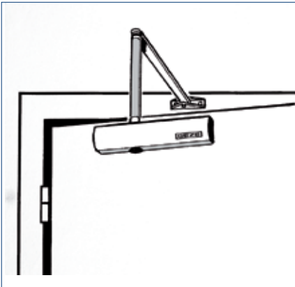
TS 4000 door leaf installation/hinge side
