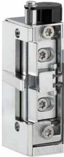
The SILENCE electric strike for fire protection doors FT201SF dampens the swing-back of the strike latch and therefore ensures that it falls back quietly into its starting position. It is perfectly suited for use on fire protection doors in which there should be no swing-back noise due to local conditions.
