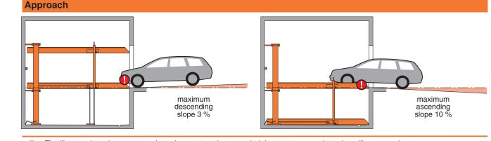
The illustrated maximum approach angles must not be exceeded. Incorrect approach angles will cause serious maneouvring & positioning problems on the parking system for which the local agency of KLAUS Multiparking accepts no responsibility.
