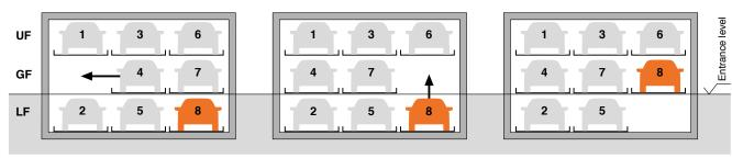
For driving the vehicle off platform No. 8 the ground floor parking platforms are shifted to the left
