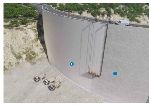
1 Substrate 2 Waterproofing layer TPO Aqua 2.5 Geo
