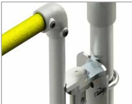
**1.** Open up gate assembly and fit U bolts, washers and nuts. Align fixing plate, ensuring top rail of gate is level with guardrail.
