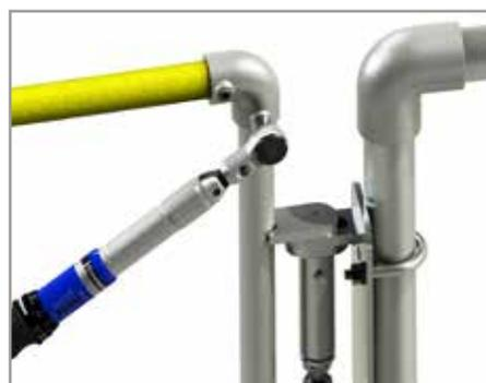
**6.** Replace tubular gate, and tighten grub screws to 39 Nm.
