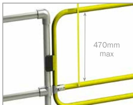
**9.** Ensure mid rail is level, and gap between top of gate and mid rail is not greater than 470mm, and torque clamps to 19 Nm.
