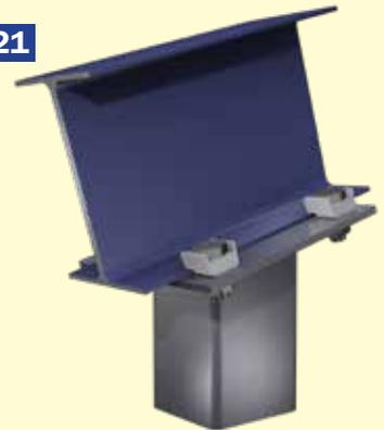
Column end plate to sloping I-Section
