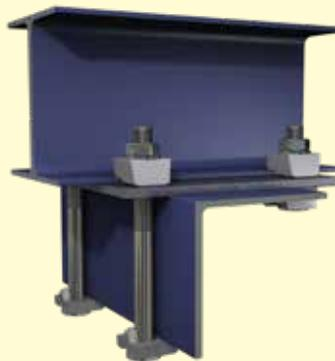
Angle section below an I-Section at 90 degrees
