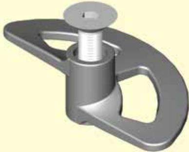
**THE FLOORFIX HT** has been developed following customer feedback to provide a fixing with increased functionality to suit a wider range of applications. **FLOORFIX HT** is designed to fix flooring plate to supporting steelwork from the topside only without the need for time consuming on site drilling, tapping, bolting or welding. It works on a cam mechanism that can be operated using a basic hexagon key drive.
