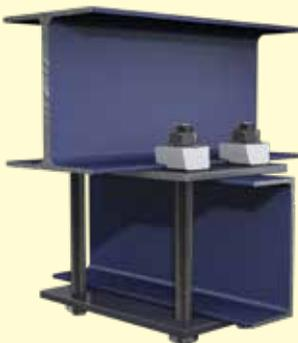
Channel section below I-Section at 90 degrees
