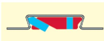
**1.** Select the correct position for the grub screw to suit decking profile as shown on the left Position 1 or 2.
