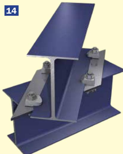
I-Section to I-Section with an angled cross over
