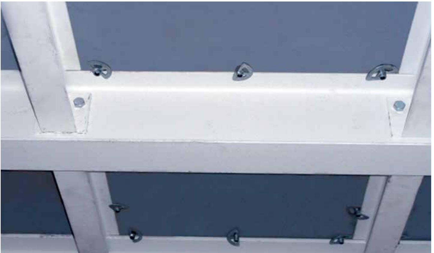
The **FLOORFIX HT** (High Tolerance) was used to secure the chequer plate flooring onto to the supporting steelwork from the top side only requiring no access to the underside and no need to drill or weld the supporting structure. The **FLOORFIX HT** allows for steel erection tolerances of plus and minus 6mm without compromising the integrity of the fixing.
