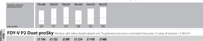
FDY-V/U P2 Duet proSky Window with safety double glazed unit. Toughened outer pane. Laminated inner pane. U-value of window 1.3 W/m²K
