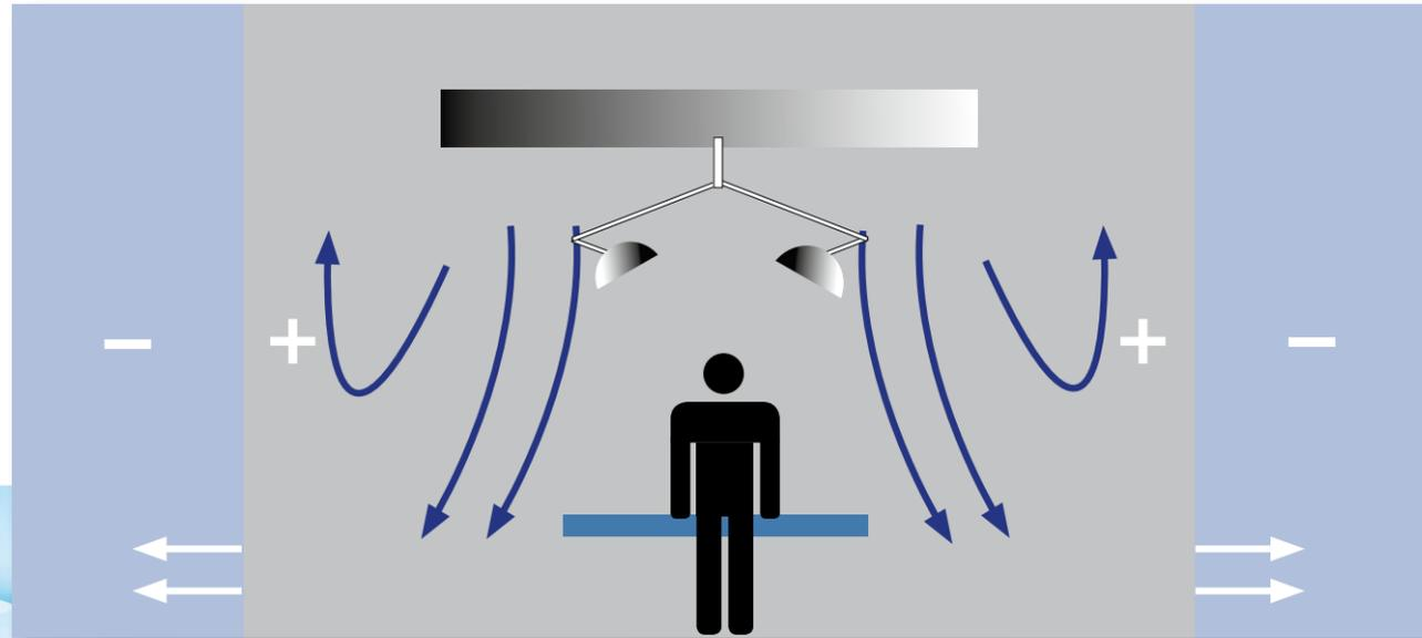
In addition to the clean room and various room air flow laboratories, you have reconstructed an operating theatre in your institute and investigated how the stability of laminar or low-turbulence airflows can be maintained under the specific influencing variables.
