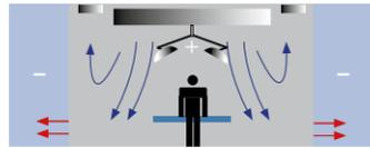
Low-turbulence laminar flow
