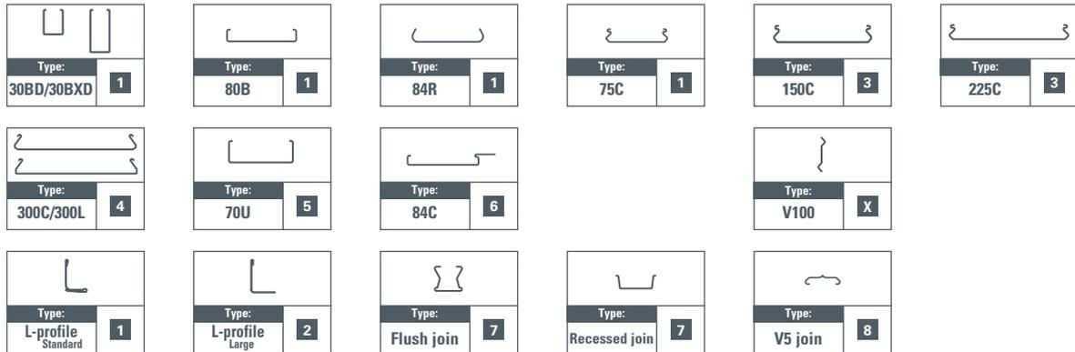
Flush-, V5 join profile only for 84R. Recessed join profile only for 80B.
