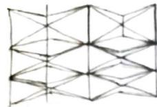
HeartFelt® Origami is based on the principle of a stiffening technique that requires less material and a felt product that has special acoustic properties.
