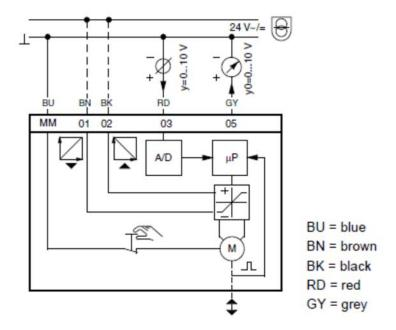
The direction of response to the 0-10V control signal is reversible.
