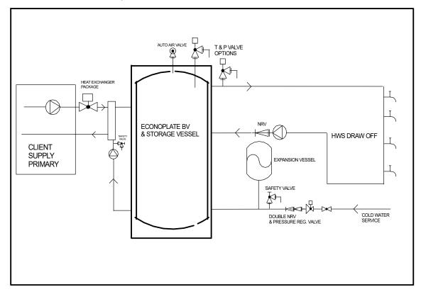
Typical Schematic of Econoplate BV Model EE on a Combined Heating & Hot Water System with Unvented Cold Feed.
