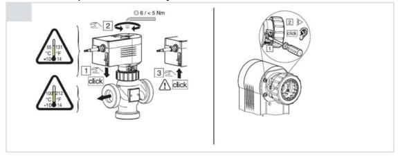
When replacing the actuator the following procedure should be followed. To remove:
