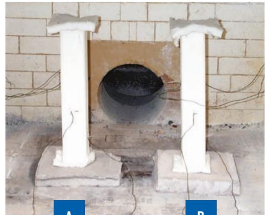
Steel columns applied with FIRETEX<sup>®</sup> FX range, before fire test burn
