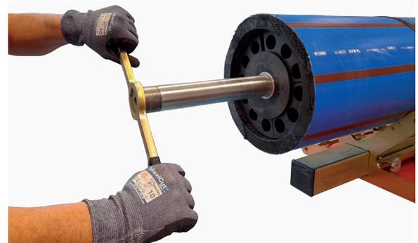
2. Adjust the collet by twisting the mandrel shaft clockwise until the mandrel becomes secure in the bore of the pipe and tighten with the mandrel spanner. To achieve the correct alignment parallel to the pipe bore, a joggling action in all directions is required. The collet also acts to re-round the pipe so check for gaps between the collet and the bore of the pipe.
