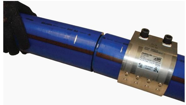
5. Ensure the shells are flush with the pipe ends or for the straight coupler, centre the shell between the depth penetration marks. The fitting is ready to be tightened. Set the torque wrench to the value indicated on the label of the shell.
