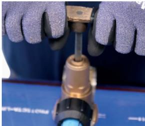
*NB. You should feel growing resistance before the cutter turns easily and then stops. It is normal to get a slight discharge of water during this operation.*
