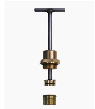
7. Fit the liner insertion head to the outlet of the ferrule. Open valve and push the stem down until liner engages with main (may require some additional force to deploy liner fully into main).
