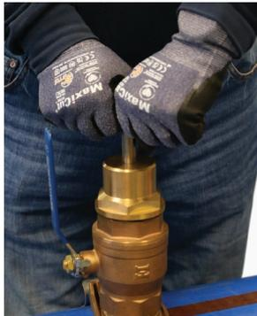
8. Withdraw the liner insertion head stem until the carrier is fully withdrawn into the liner insert head. Close the ball valve and remove the liner insertion head.
