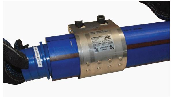
4. Offer up the second pipe end onto the insert and push the pipes together, ensuring both pipes are up against the pipe stops of the insert and correctly aligned on the pipe.
