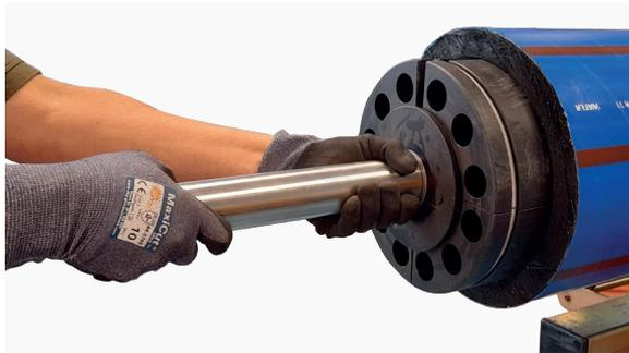
1. First mark the required length of pipe to be scraped (see table on page 11). Ensure that the correct size collet for the pipe to be scraped is fitted to the mandrel. Adjust the collet by twisting the mandrel shaft anti-clockwise until it achieves its smallest outside diameter.
