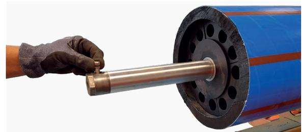
3. Once the mandrel is secure and is parallel with the pipe bore, screw down the quick release screw to its full extent (about one and a half turns) using the adjuster, which is stored at the base of the tip arm support block.
