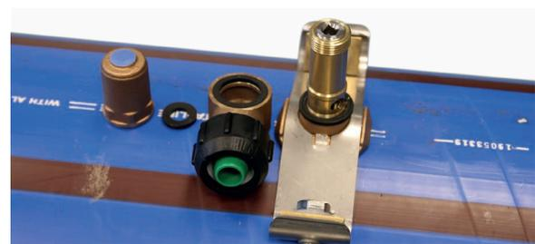
1. Unscrew body top and outlet banjo ensuring all seals are retained and set aside, which is only applicable on mains 200mm and above. Ensure that the sealing O-ring is in place under the upper ferrule strap (take care not to damage this on the protruding sleeve).
