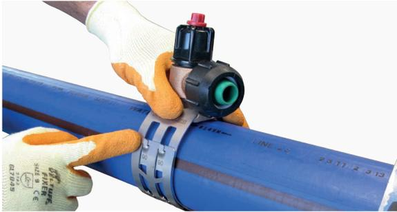
3. Tighten the strap bolt with a 13mm socket wrench or spanner to 12-14Nm of torque.
