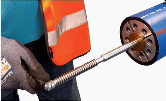
4. Hold the expanding collet and rotate the mandrel anticlockwise until the collet is a light interference fit in the pipe bore.
