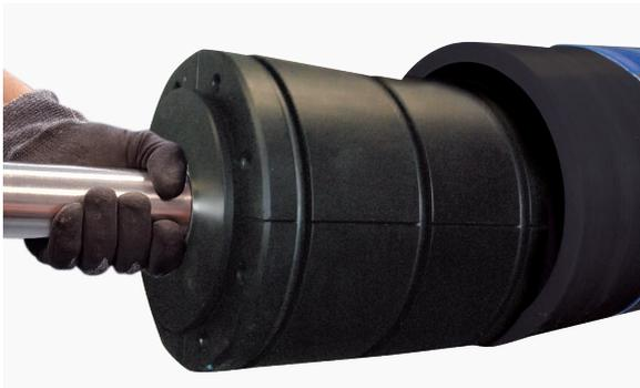
9. Remove the collet and mandrel from the pipe. The collet should be removed to a clean dry and safe area. If there are any areas of pipe that have not been prepared properly, then the hand scraper should be used to complete the preparation process.
