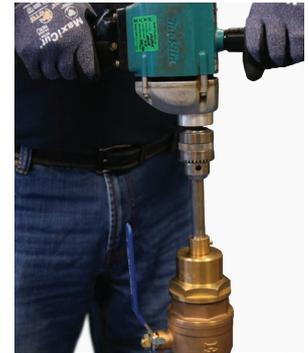
5. Disconnect power supply and remove drill from stem. Withdraw stem, until the cutter is fully returned into the drill head and fully close the valve (handle is horizontal to valve) before removing the drill head from the outlet of the ferrule.
