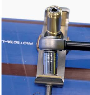
3. Ensure pre-cutter is installed, and replace outlet banjo with large seal top and bottom.
