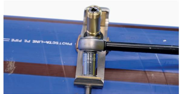
2. Fit strap squarely on main and tighten bolts to a torque 20Nm - 24Nm. Make sure both bolts are tightened evenly.
