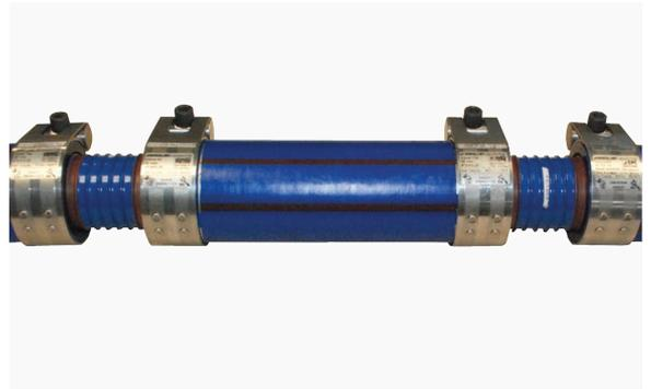
7. Tighten the hex socket head bolts until the set torque is achieved in each bolt. The pipe will relax after the set torque is achieved, so after a minute or more, retighten the bolts to the set torque. Repeat until less than a quarter turn is needed to reach the set torque.\*
