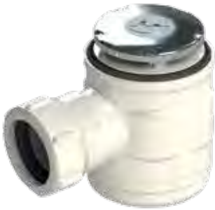
Waste trap** comes in four sizes: 19mm, 50mm, 90mm and low depth 90mm.
