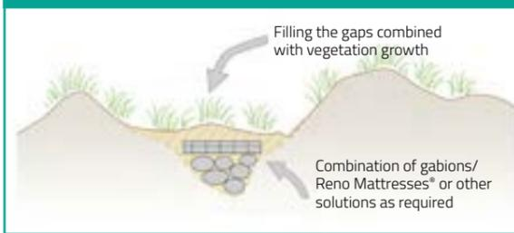
Breakwaters and Groynes are designed to reduce the effects of waves and currents approaching the coast. They can be submerged or emerged and in the case of breakwaters can be either attached to the shore, or positioned offshore.
