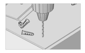
When installing a ramp-back profile over a resilient floor covering, fit the covering before placing the stair nosing profile onto the step to mark off the position of the holes. Drill according to the substrate: pilot holes in timber, holes for plastic plugs in solid surfaces.
