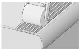
Finish with a seam roller to ensure complete contact along the entire length of the now joined pieces.
