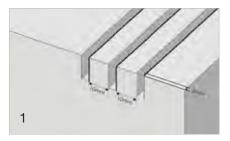
Rebate the step as required for the dimensions of the chosen profile with an allowance for the adhesive and for the profile to sit 2mm above the step in the finished installation.
