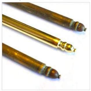
The image above shows old tarnished rods before and after re-polishing .
