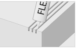
Apply a bead of adhesive to the centre of each of the rebates. The amount of adhesive should be sufficient to spread across the base and part way up the walls of the profile but not ooze above the top surface when pressed into position.
