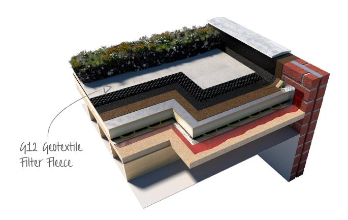
A needle punched polypropylene filter fleece for use as a protection and filter layer in green roofs.
