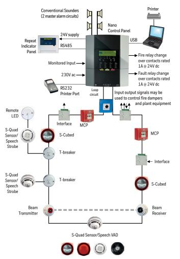
Nano is compatible with Vigilon's range of advanced detection and alarm loop devices
