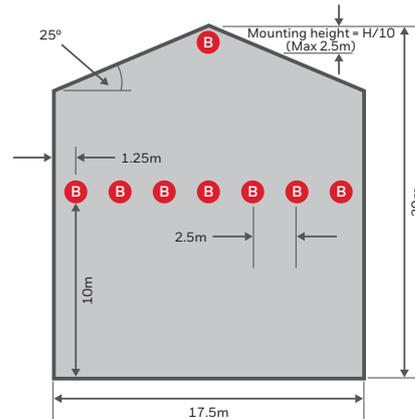
One beam detector covers 18.75m using extra % allowed due to angle of roof.
