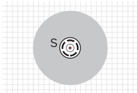
Where air is forced through a perforated ceiling, the detector should be mounted on a solid baffle with a minimum diameter of 1200mm
