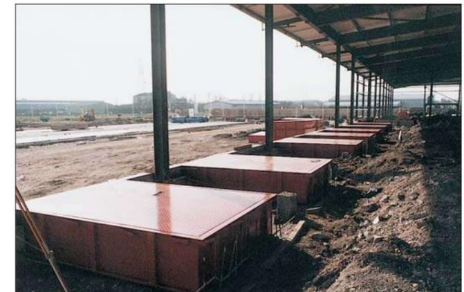
Levellers in heavy-duty fabricated steel pouring pans
