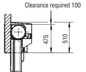
Vertical section - with barrel and motor cover
