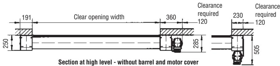
Section at high level - without barrel and motor cover
