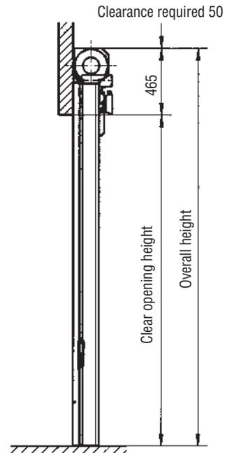
Vertical section - without barrel and motor cover
