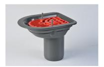
ACO Balcony outlets are designed to be installed against an abutment wall and permit the introduction of successive rainwater pipes discharging from higher level balcony areas. Balcony outlets are suitable for connection to pipes of 82.5mm and 110mm outside pipe diameters.
