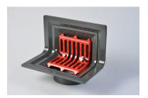
ACO Two Way outlets are located at the junction between flat roof and parapet wall providing "through the wall" drainage to external rainwater pipes and hoppers. Outlets are parallel threaded for connection to taper male, screw threaded adapters to ensure a completely watertight connection to pipes with 55mm, 82.5mm and 110mm outside pipe diameters.
