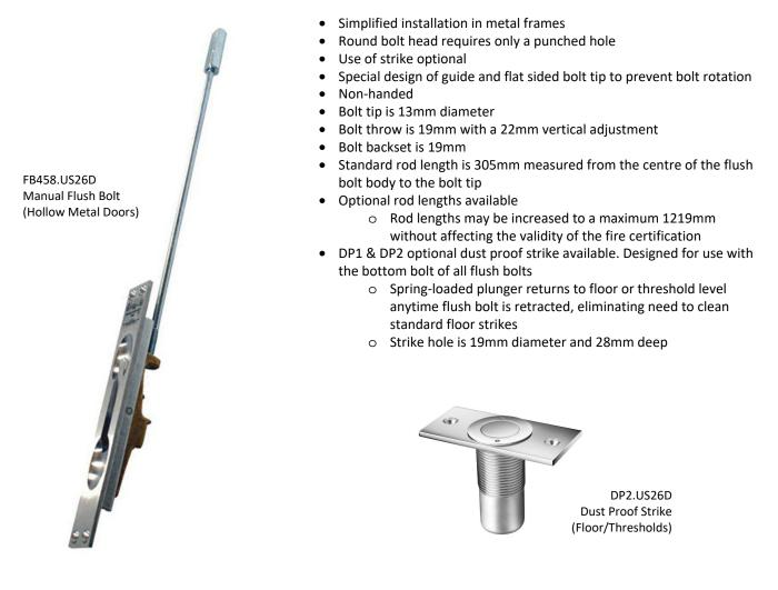
Tested and assessed as suitable for use with metal based doorsets tested to the requirements of EN 1634-1:2008. Assessment report WF No.335640 for up to 240 mins.
