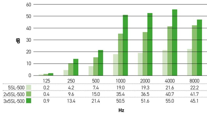
The diagrams illustrate the increased sound absorption levels when close-coupling up to three individual 0.5m lengths of rigid duct attenuators, thus reducing noise levels by up to 55dB.
