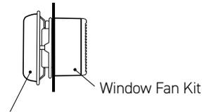
Weather cowl can replace the external grille and window sealing plate
