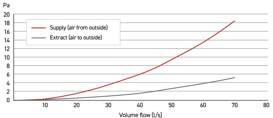
Performance data for double airbrick (code 905) with adapter (977)
