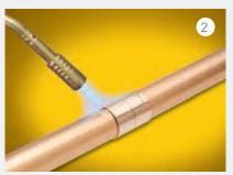
**2.** Insert the tube into the fitting until it reaches the tube stop, then wipe off any excess flux. Heat the assembled joint evenly on all sides.
