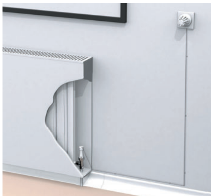
2. The new radiator valve is attached to the pipe work and the tailpiece extended and connected to the valve.
