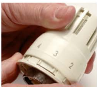
2. When engaged, the tool is twisted and pulled down to remove the inner ring. The head is lifted and rotated so that the plastic arrow above the thermal ring aligns with the required temperature setting number.
