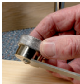
6. The standard thermal ring can be unscrewed and removed from the tool and the 'C' end of the tool used to tighten the ring onto the valve.
