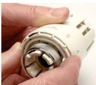
3. The inner ring is re-inserted into the head ensuring that the lugs on it are not aligned with the notches.
