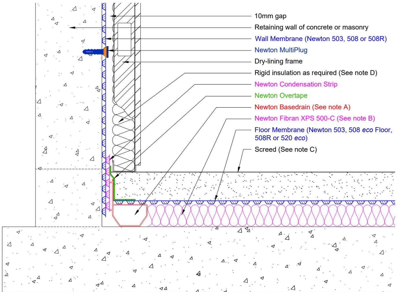
This detail assumes that the raft is in good condition - constructed to BS EN 1992 (Eurocode 2), and that the structure as a whole is of sufficient mass and quality to resist heads of water pressure as required by BS8102.
