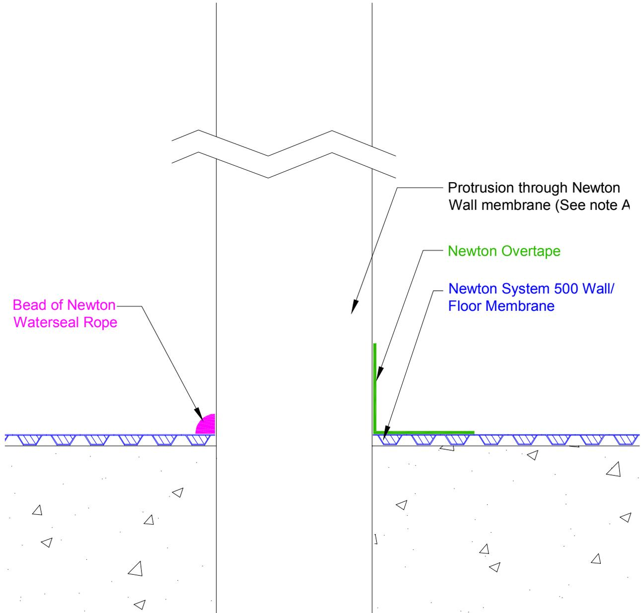
This detail shows a protrusion, such as a pipe or steel, through the Newton System 500 Wall/Floor membrane, showing sealing with Newton Waterseal Rope or Newton Overtape as options. This detail should be used in conjunction with Newton System 500 drawings prefixed RA or SA.
