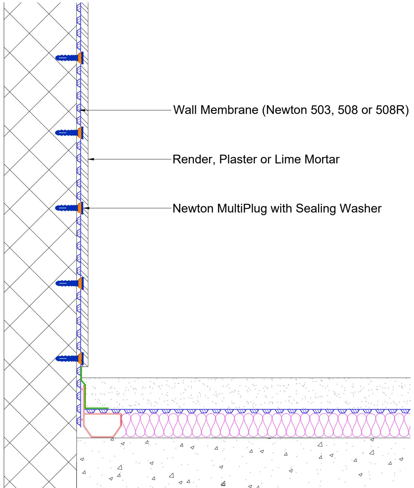
NEWTON CDM - CAVITY DRAIN WATERPROOFING SYSTEM
