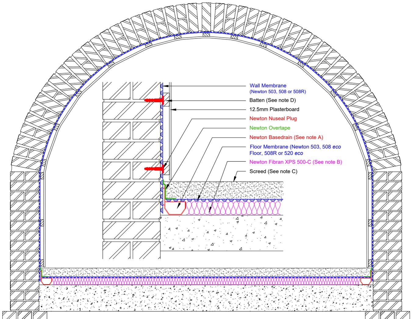
This detail assumes that the slab is in good - constructed to BS EN 1992 (Eurocode 2), and that the structure as a whole is of sufficient mass and quality to resist heads of water pressure as required by BS8102.
