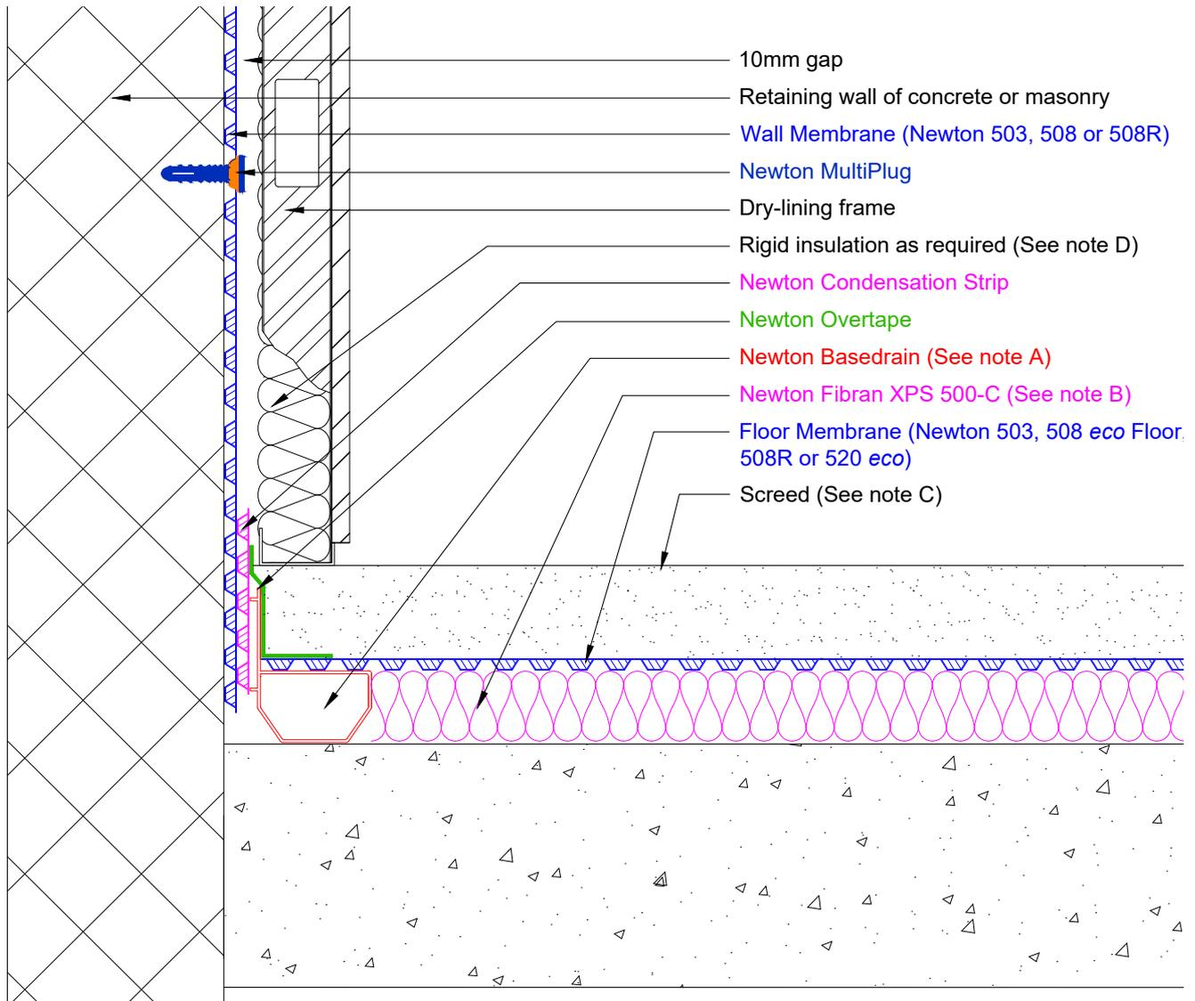
This detail assumes that the slab is in good condition - constructed to BS EN 1992 (Eurocode 2), and that the structure as a whole is of sufficient mass and quality to resist heads of water pressure as required by BS8102.
