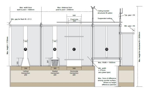
Sample elevation to illustrate available transaction gap types, upper fixing styles and system limitations.
