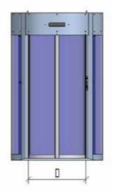
1500 x 1700 x 2400 mm (A x B x C) Passage width: 900 mm (D) Passage high: 2000 mm (E)
