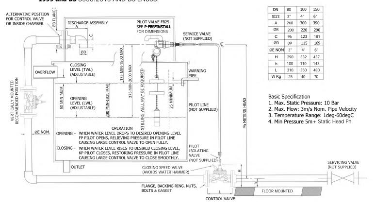
Control Valve Location There are four options for the mounting of the Control Valve -
