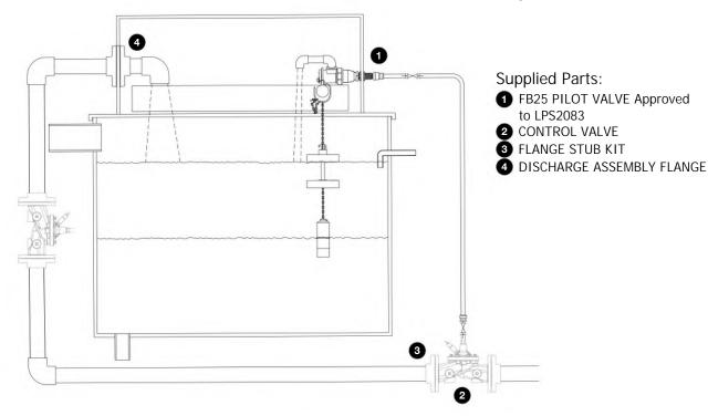
FP Type Valves offer a flexible solution to the installation of large Float Operated Valves in sprinkler tank systems
