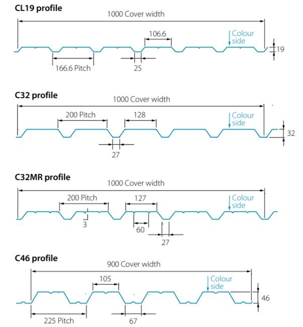
Note: All measurements in diagram are in mm.
