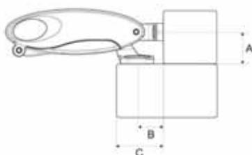
A = Fixing centre to frame 25mm
