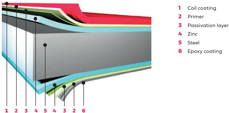
Standard thicknesses of the coil coated steel sheet are 0.5 and 0.6 mm.
