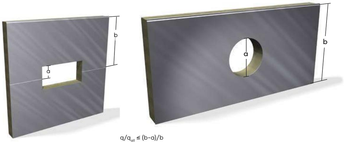
If the degree of cut-out exceeds the ratio  $q/q_{all}$ , the load is either to be transferred to adjacent panels in accordance with figure 14 or, if this is not possible, to be directed on the load-
