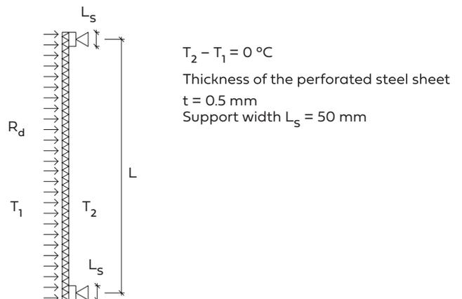
Figure 10. Spans for Paroc Panel System acoustic panels in single-span internal walls without temperature gradient.
