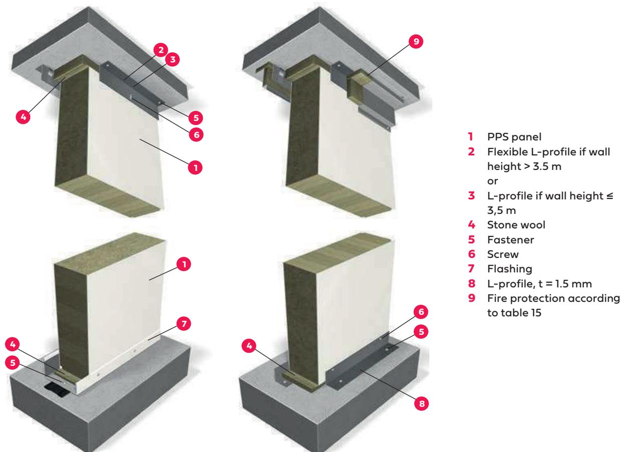
Panel joint in horizontal installation.
