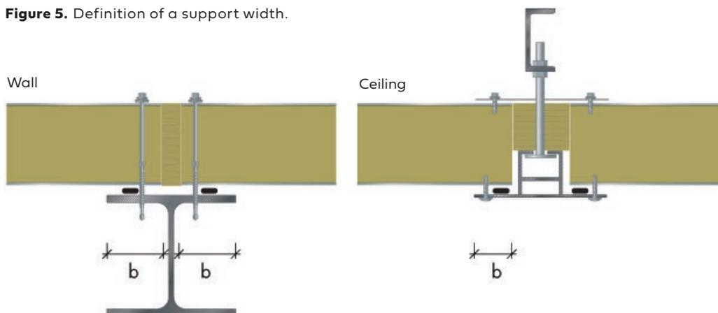
When support width  $L_s$  is known the design value of the support resistance of panel  $F_{Rd}$  at the ultimate limit state can be calculated as follows:
