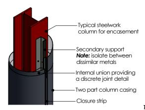
Isometric View (on typical butt joint with internal union)
