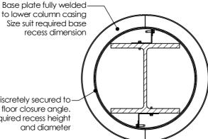
Recessed collar discretely secured to base plate flange and floor closure angle.
