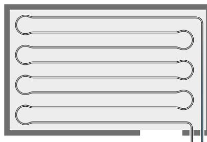
Pipe is laid in parallel runs up and down the room length, with loop turns at each end. Hep<sub>2</sub>O panel products all use the serpentine pattern and it can also be used with staples.
