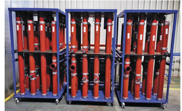
Small improvements in productivity add up to large savings for the contractor. These lovely looking units are destined for 21 Moorfields in Central London, a new 21-floor building requiring **370** of these pre-assembled cast iron above ground drainage and soil systems. The beauty of them is they are pre-assembled at our Telford factory and delivered ready to install on site, saving the installer money and reducing the install time by up to **60%**.
