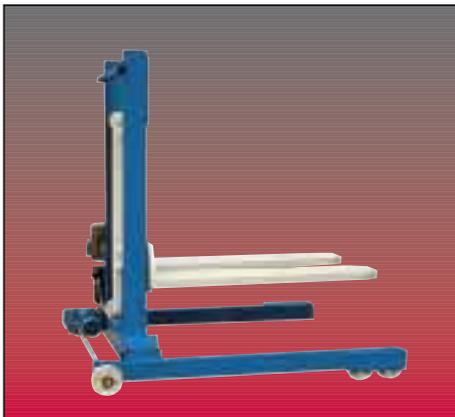
A special type of pallet lifter with powered wheels for use on rails. It has a capacity of 1,500Kgs and a vertical stroke of 600mm. It can be used as a combined lift / transporter on a production line.
