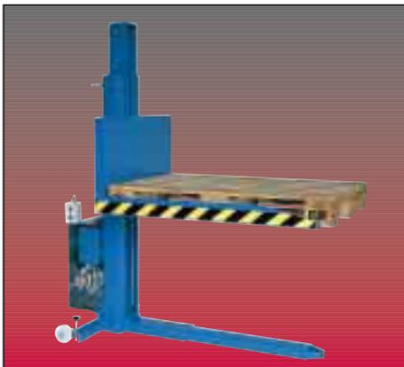
A 1,000Kg Euro-pallet lifter. Vertical stroke of 800mm. A low closed height of 80mm, allows loading by a standard manual pump truck.
